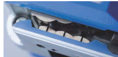
The sealing mechanism of the E-Series Tool
